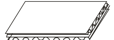
Liner + MD wave + liner + CD wave + liner
