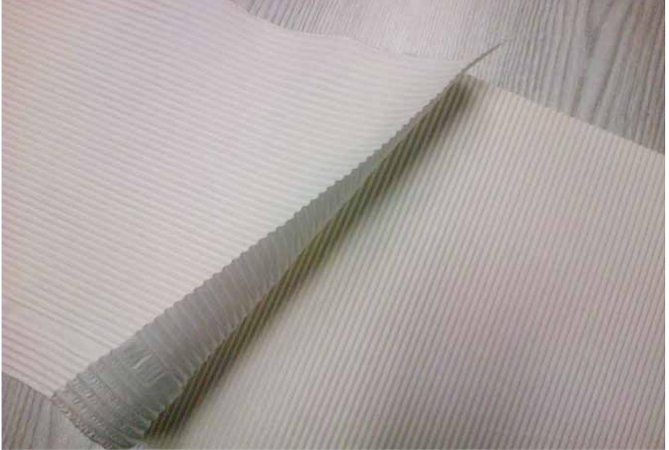
Novel longitudinally corrugated web as stable wave obtained by the Papermorphosis process (left), combined to traditional corrugate (right)
